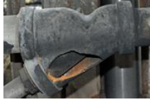
आकृती १. Left, schematic for २०१९ incident, (CSB Report No. २०१९-०२-I-TX). Right, ruptured strainer (CSB), from red circle in schematic.
