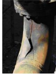
आकृती २. Left, schematic for २००७ incident, based on CSB Report No. २००७-०५-I-TX. Right, cracked inlet elbow (CSB)
